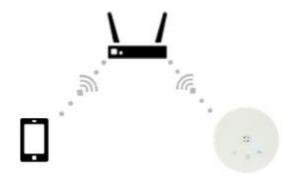
If you have a wireless router, you can connect LED controller box to router first. Then, connect phone (WIFI) to router and open app to control LED controller box.
