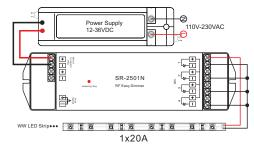
2)Receiver Connection Diagram for Multiple Units
